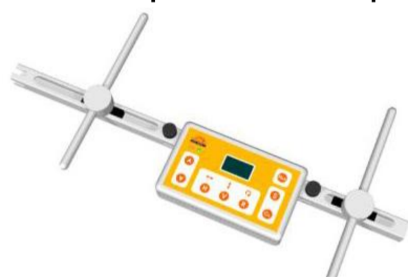
Horizon (Society for Research on Sitting Posture Measurement) measures sitting posture in accordance with ISO16840-1:2006.
