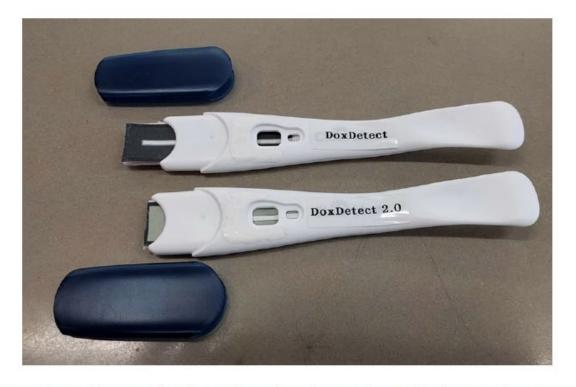
**Figure 1.** Prototype point-of-care devices for the detection of chemotherapeutics in urine. Two different versions of the printed wax test strip at 25% grayscale (top) and 50% grayscale (bottom) can be observed, surrounded by a dark black border to limit sample loss from the test strip.
